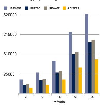
Data assumes nominal conditions, 6000 operating hours per year, 0.12€/kWh utility rate, compressor generation efficiency of 5.5 kW/m³/min.
